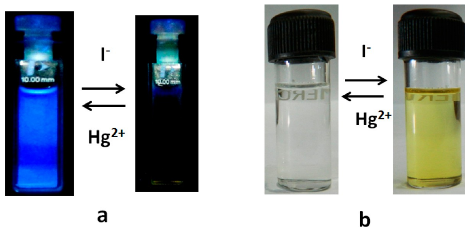
Figure 1. Color of the PPT solution in a 4:1 THF/water solution under (a) ultraviolet (UV) light and (b) the naked eye.
